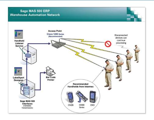
The Warehouse Automation network efficiently transfers information between Sage MAS 500 and wireless handheld devices in the warehouse to streamline picking, packing, shipping, and receiving.
